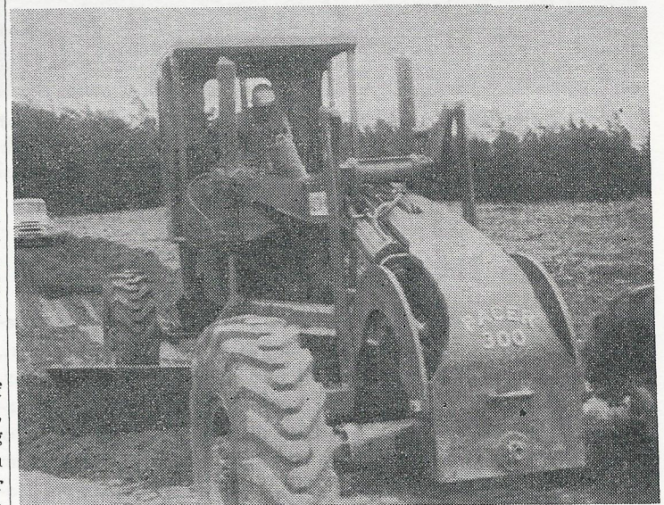
Above you see the new Austin-Weston Road Grader. The grader, which is a Pacer Model 300, replaces our former grader, which was war-time surplus.
