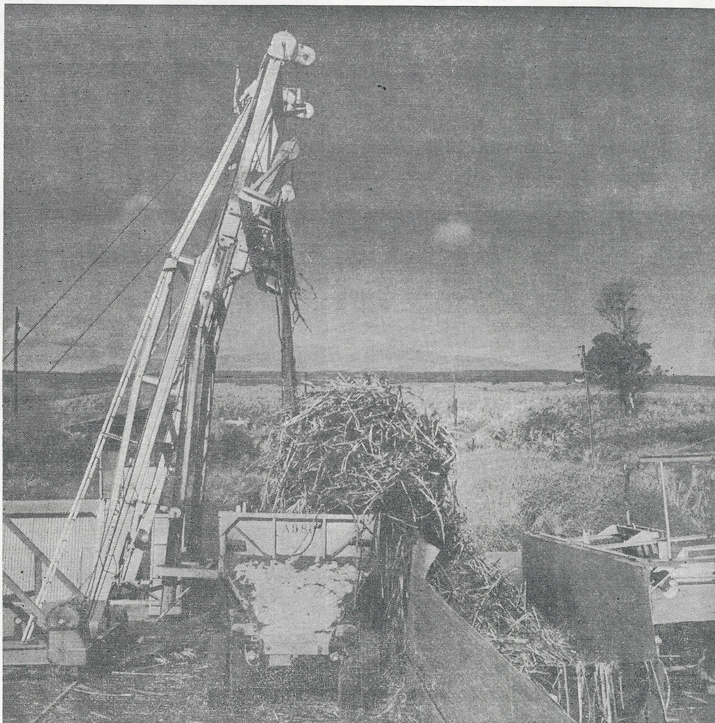
KAMAE UNLOADING STATION feeds the hungry mill its diet of sugar cane. The unloaded cane travels down to the mill at a steady pace via a flume. A much earlier version of this station is pictured above.
